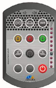
Control panel with Public Address function - 32710
